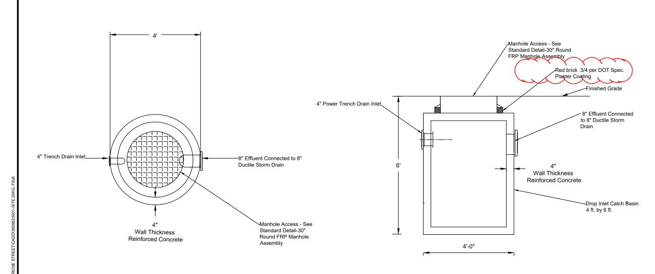
Catch basin must be rated for a minimum of H-20 loading
